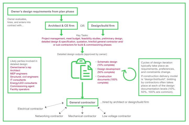
Using a "design/bid/build" construction delivery model, construction general contractors and subcontractors are chosen through a process of bidding at each of the design documentation completion levels.
